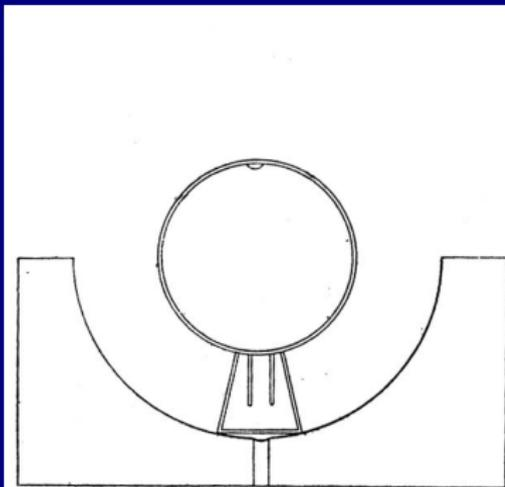
FIG. 1.—Section of Mr. Campbell's original Sunshine Recorder.
