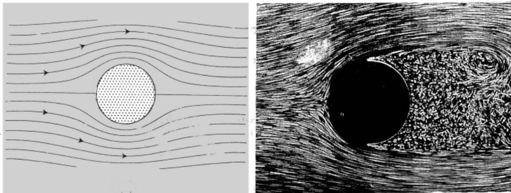
*Fig. 9.1 Flow past a circular cylinder for (a) a hypothetical fluid with zero viscosity, (b) a real fluid with very small viscosity  $\mu$ . (from van Dyke 1982).*
