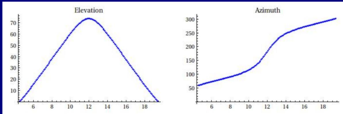
Figure : Solar elevation and azimuth for observation at  $40^\circ\text{N}$ .
