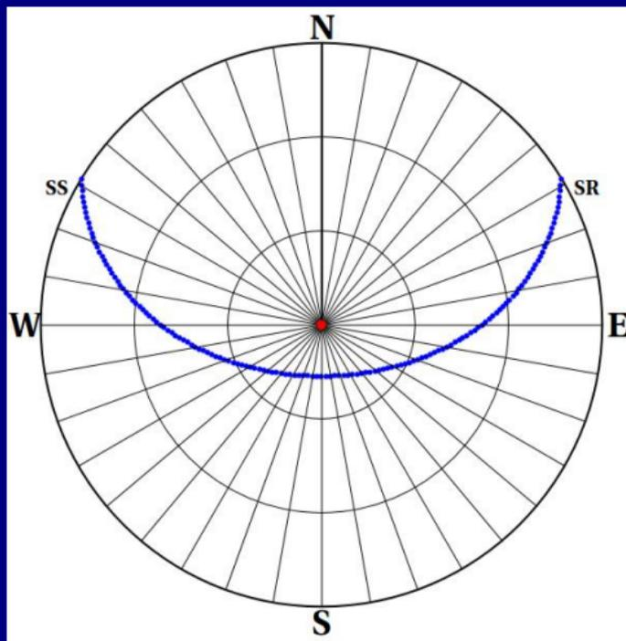
Figure : Path of the Sun for observation point at  $40^\circ$ N.
