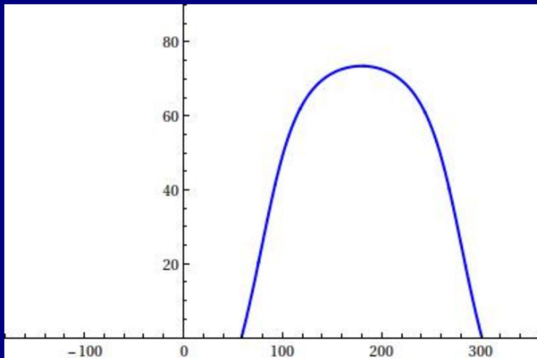
Figure : Elevation versus Azimuth for observer at  $40^\circ$ .
