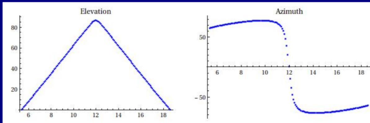
Figure : Solar elevation and azimuth for observation at  $20^\circ\text{N}$ .
