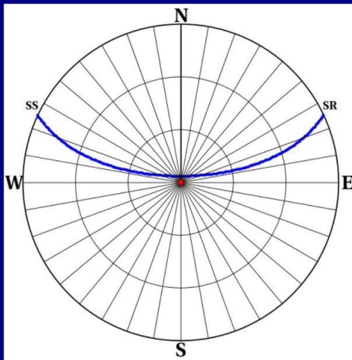
Figure : Path of the Sun for observation point at  $20^\circ$ N.
