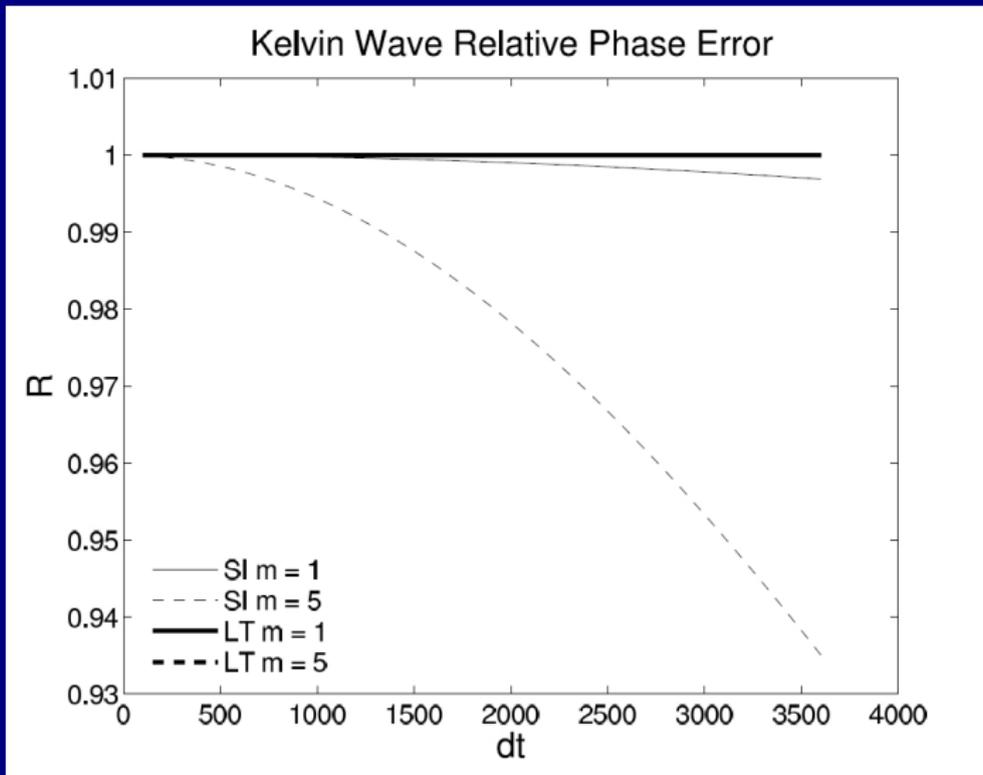
**Relative phase errors for semi-implicit (SI) and Laplace transform (LT) schemes for Kelvin waves  $m = 1$  and  $m = 5$ .**
