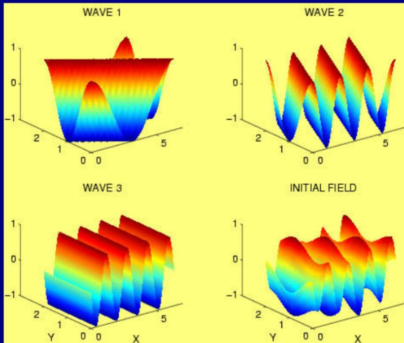
**Components of a resonant Rossby wave triad**
