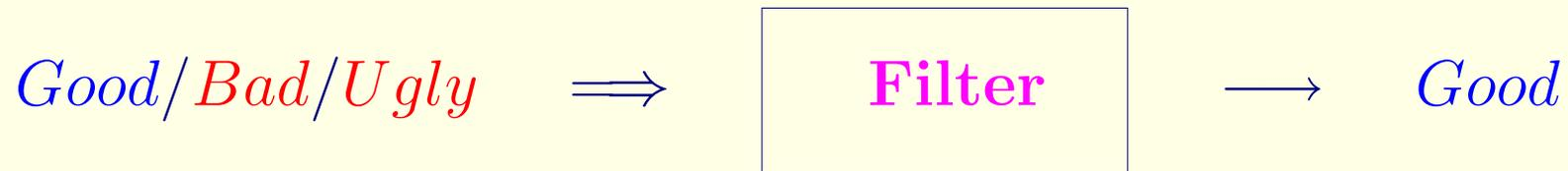
Suppose the input consists of a low-frequency (LF) signal contaminated by high-frequency (HF) noise. We use a low-pass filter which rejects the noise.
