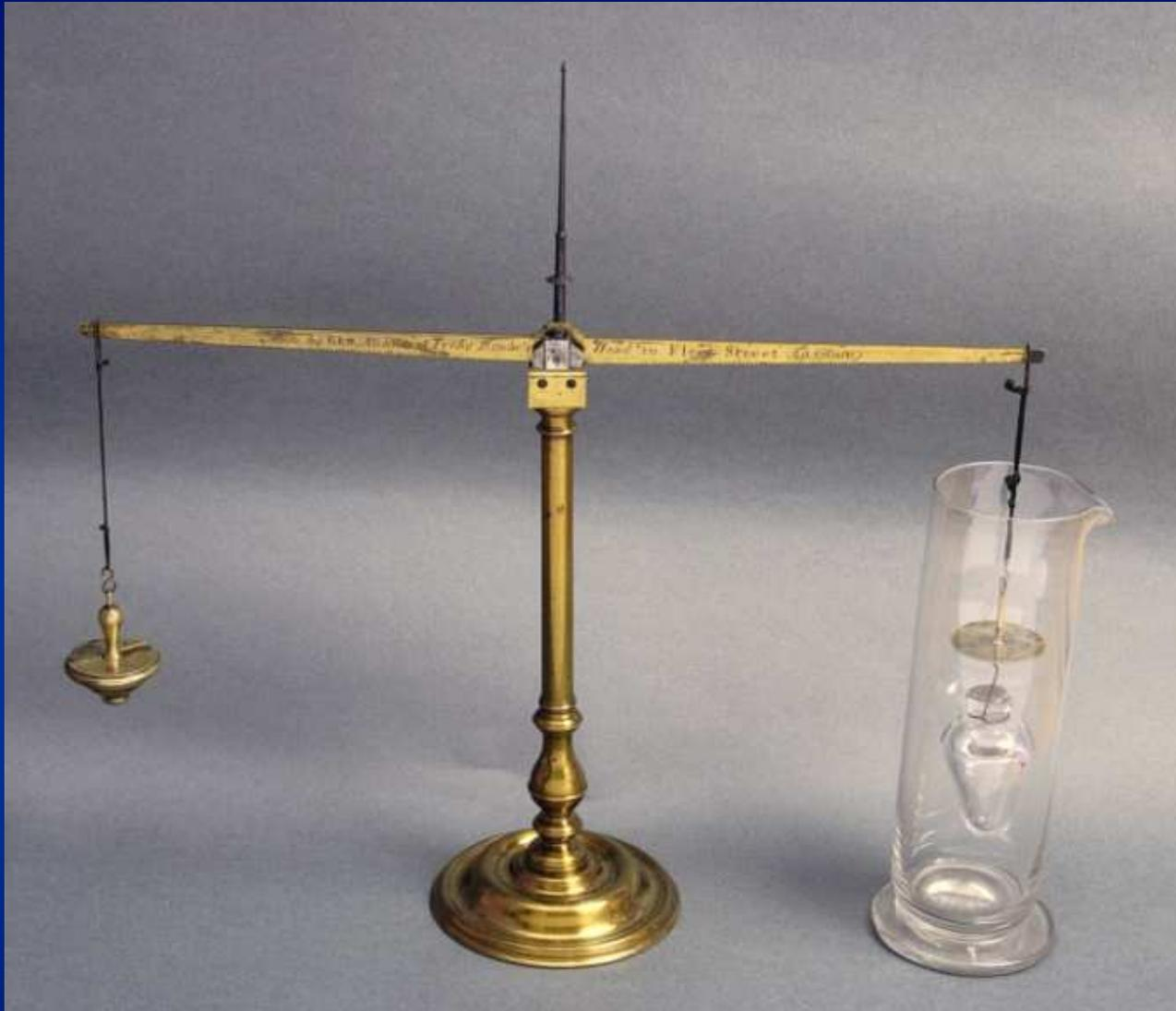
**This balance can be used to determine the specific gravity of solids by weighing them in air and in water.**
