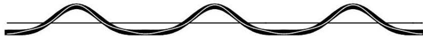
Figure 3: Form of the Stokes wave, with sharpened crests and flattened troughs. Thick curve: second-order approximation. Thin curve: third-order approximation.
