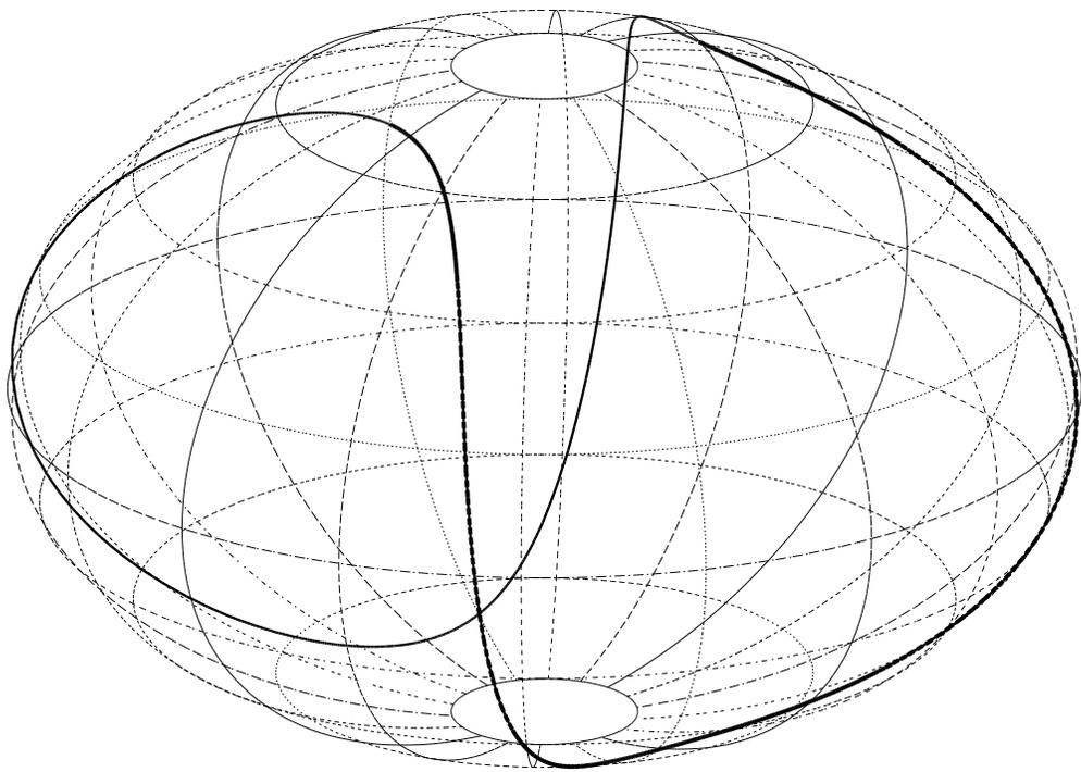
Figure 3: The Tennis Ball curve, the intersection of two offset elliptic cylinders, and also of a sphere and hyperbolic paraboloid or hyper.
