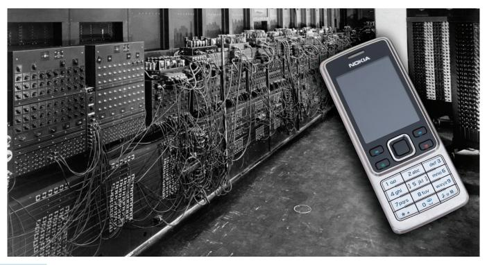
Figure 1: ENIAC v 'PHONIAC' – The 'PHONIAC' (a standard Nokia 6300 from 2008) could compute a 24-hour forecast in less than one second, compared to the 24 hours it took the ENIAC, circa 1946.
