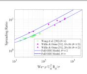
Experiments: Willis and Orme use a head-on collision of two droplets... equivalent to  ${\rm CA=}90^{\circ}$ . Wang et al. use an engineered superhydrophobic surface with  ${\rm CA=}180^{\circ}$ .
