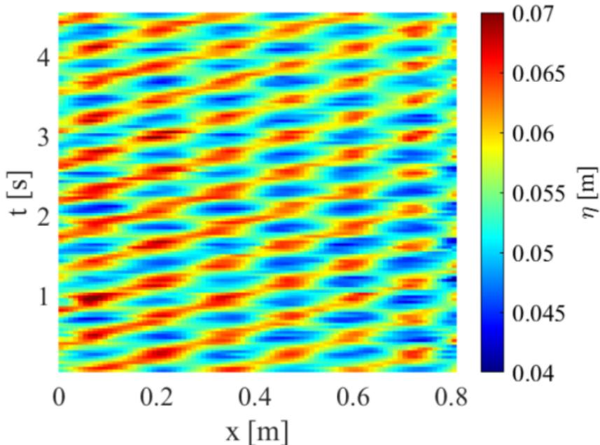
Evidence of superposition of standing wave (reflection) and travelling wave (outgoing / absorbed) BC.
