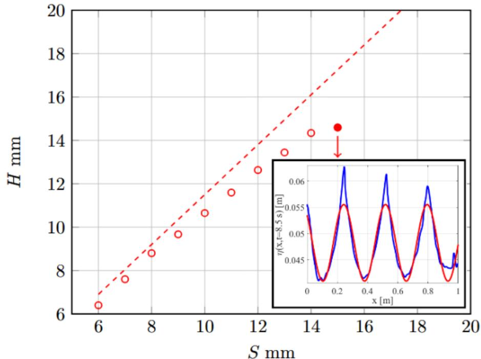
Dashed line: linear theory; dots: DNS. Increasing  $S = 2f_0$  means waves become non-linear.
