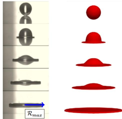
Droplet impact study. Left: high-speed camera. Right: OpenFOAM simulations. Credit: Conor Quigley. Parameters:  $\text{Re} = 1700$  and  $\text{We} = 20$ .
