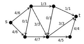
(g) The residue network is then as follows. It is not possible to find a directed path from source to sink, so the previous flow was a maximum flow (with value 8).
