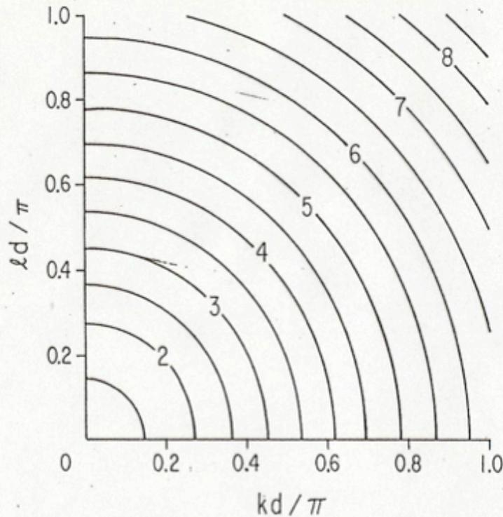
FIG. 9. Contours of the (nondimensional) frequency as a function of the (nondimensional) horizontal wave numbers for the differential shallow water equation for  $\lambda/d = 2$ , presented for comparison with Fig. 8.
