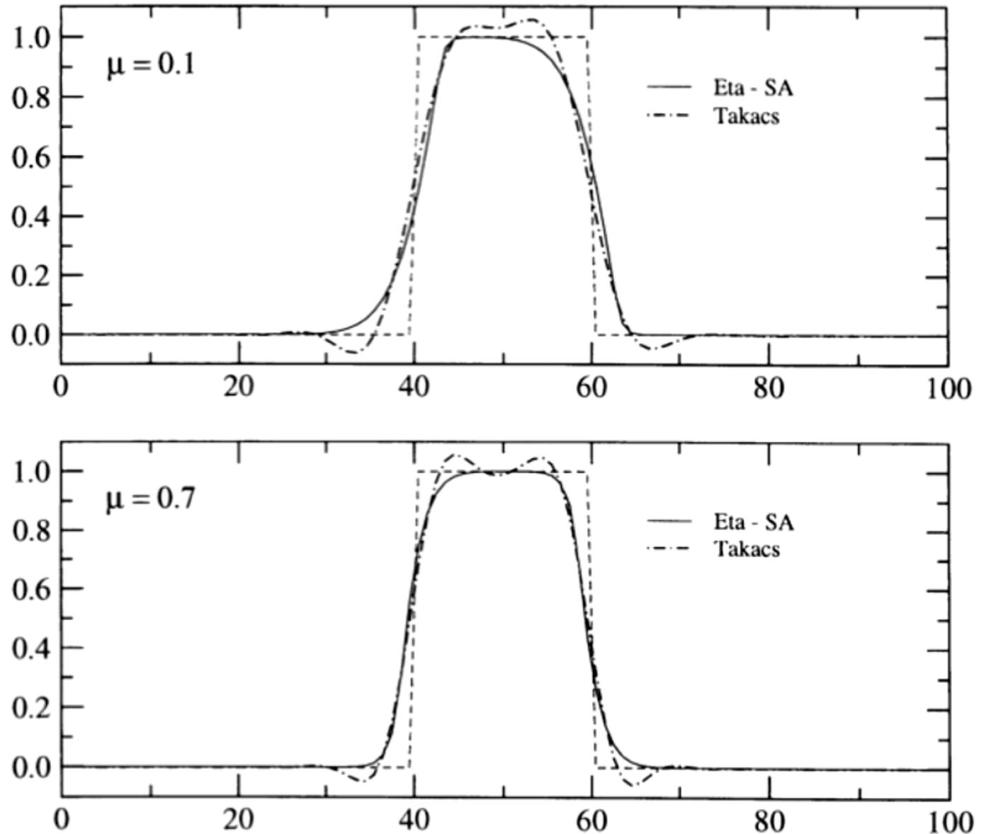
Figure 9. Same as Fig. 2, except for the Eta slope-adjustment scheme results (SA, solid line) compared against those using the Takacs (1985) third-order "minimized dissipation and dispersion errors" scheme (dot-dashed line). See text for definitions of schemes.
