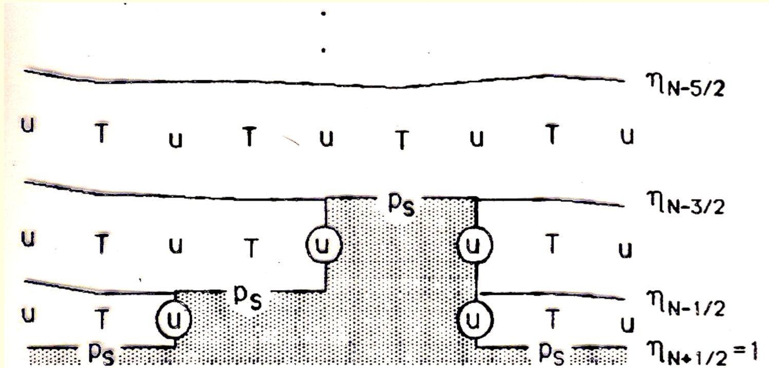
FIG. 1. Schematic representation of a vertical cross section in the eta coordinate using step-like representation of mountains. Symbols  $u$ ,  $T$  and  $p_s$  represent the  $u$  component of velocity, temperature and surface pressure, respectively.  $N$  is the maximum number of the eta layers. The step-mountains are indicated by shading.
