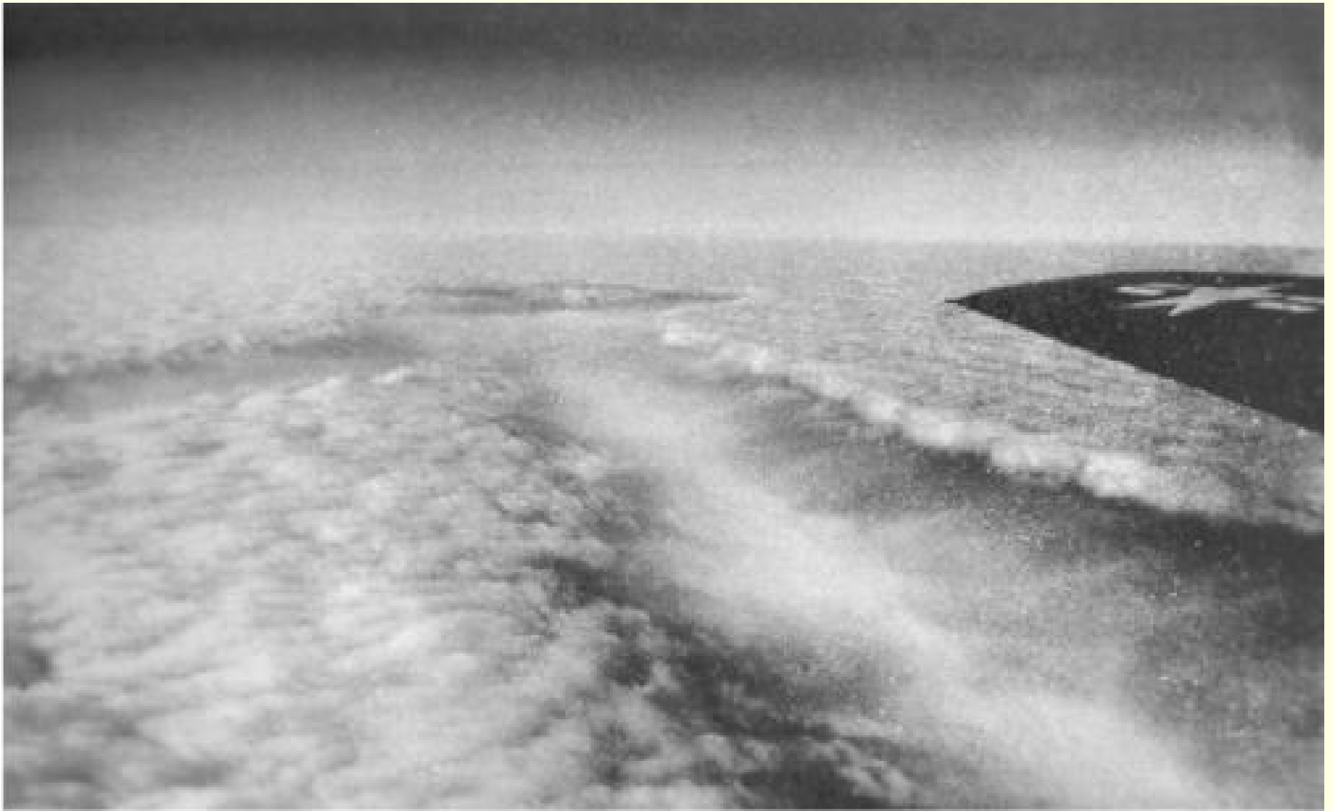
A \gamma -shaped path cut in a layer of supercooled cloud by seeding with Dry Ice (solid CO 2 ).
