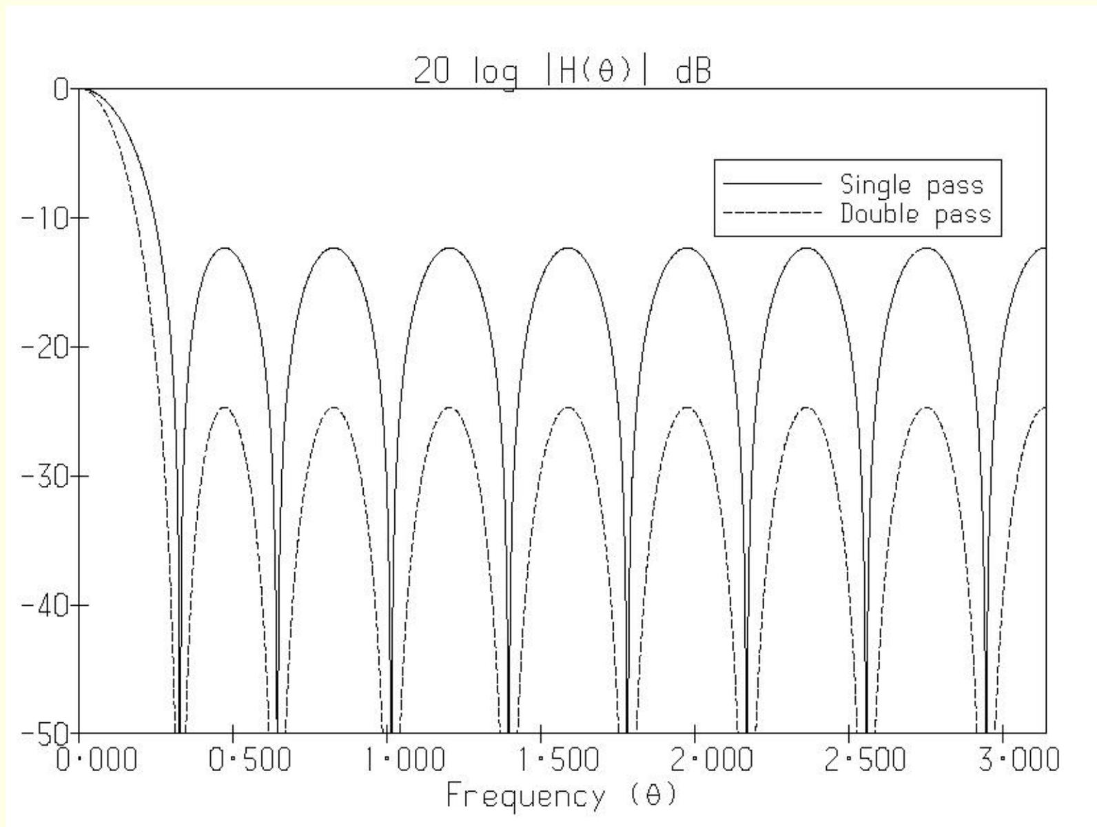
Frequency response for Dolph filter with span  $T_s = 2h$ , order  $N = 2M + 1 = 17$  and cut-off  $\tau_s = 3h$ . Results for **single** and **double** application are shown.
