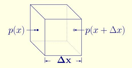
Consider a cubic box of air, of dimension  $\Delta x \times \Delta y \times \Delta z = \mathcal{V}$ .
