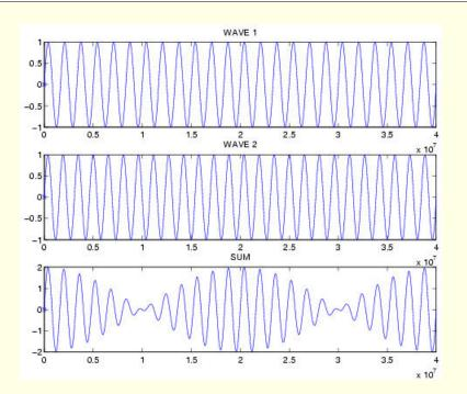
Two wave components of approximately equal wavelength. The envelope amplitude of the sum is clear.
