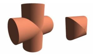
Figure 1: The intersection of two perpendicular cylinders consists of two ellipses (left). The volume of the intersection is called a bicylinder (right). **[Image needs to be redrawn]**
