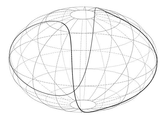
Figure 3: The Tennis Ball curve, the intersection of two offset elliptic cylinders, and also of a sphere and hyperbolic paraboloid or hyper.
