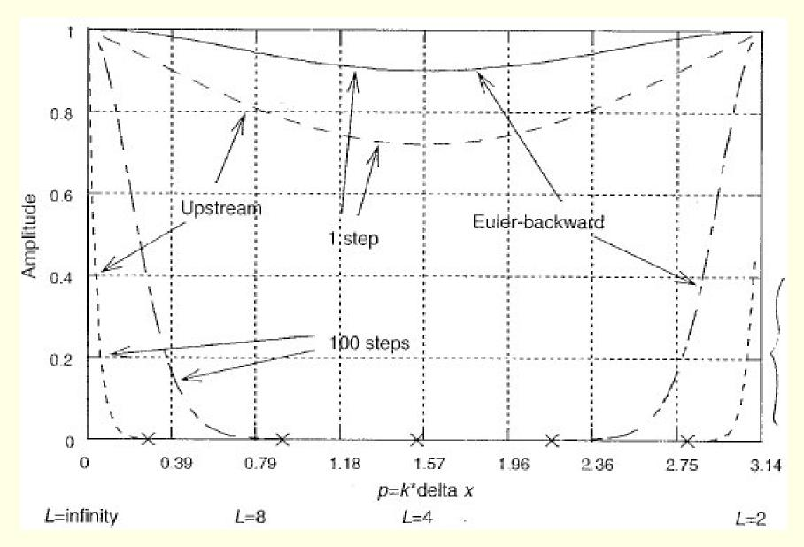
Amplification factor for the upstream scheme and the Matsuno scheme, with Courant Number  $\mu = 0.5$ . Response for 1 step and 100 steps shown. L is the wavelength in units of  $\Delta x$ .
