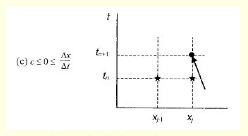
Schematic of the relationship between  $\Delta x$ ,  $\Delta t$  and c leading to extrapolation of the solution at time-level n+1.
