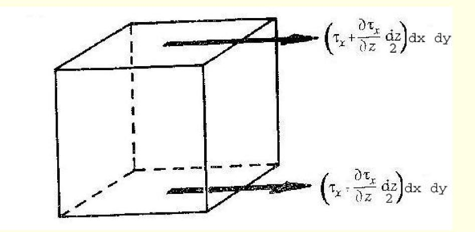
The net force is the sum of viscous forces on the upper and lower faces of the element:
